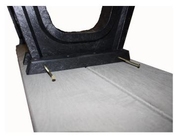
Step 1 - Lay the Assembled Bench Length upside down on a clean level surface. Place the two backless bench legs in between the 2" x 2" runners. See photo above. Step 2 - Screw 4 – 4" coated steel screws into each leg using the predrilled holes through the 2" x 2" runners. See the photo above. Repeat for both legs.
