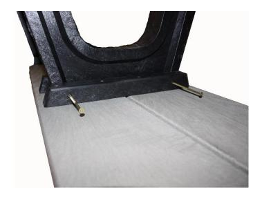
Step 2 - Screw 4 - 4" coated steel screws into each leg using the predrilled holes through the 2" x 2" runners. See the photo above. Repeat for all three legs.
