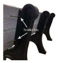
Step 5 - Screw  $4 - 4^{"}$  Coated Steel Screws into each leg using the pre-drilled holes through the 2" x 2" runners. See photo above.
