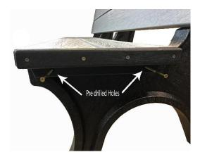
Step 3 - Screw  $4 - 4^{"}$  coated steel screws into each leg using the pre-drilled holes through the 2" x 2" runners. See the photo above.
