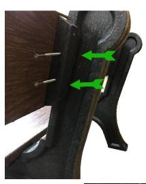
Step 5 - Screw 4 – 4" Coated Steel Screws into each leg using the pre-drilled holes through the 2" x 2" runners. See photo above.
